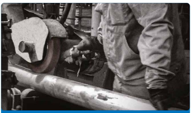
X Semi Flexible Cotton Cloth backing with Aluminum Oxide abrasive is specially designed for flap wheel with spindle and with flange. It has a flexible structure and long life.
