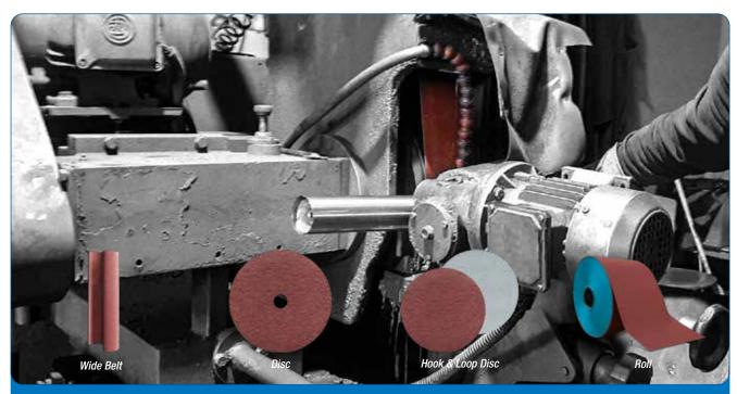
New AGYYR24 product is ideal for polishing and finishing low alloy steel, stainless steel, high alloy steel and heat resistant steel in wide belts, narrow belts, rolls and hook&loop disc; ideal for centerless grinding. YY polyester cloth backing with Semi-Open coated Compact Aluminum Oxide abrasive. Suitable for wet applications.
