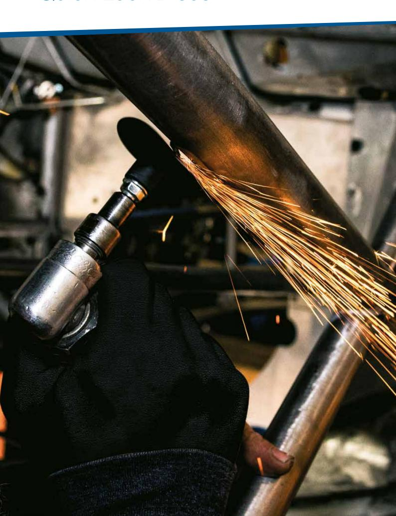
Karbosan quick lock discs are available in various specifications for polishing and sanding of small & narrow surfaces.
